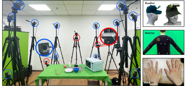
Figure 3. Capture setup. The left part shows the captured volume. MoCap cameras are circled in blue and RGB cameras in red. The right part shows in order the head marker-set for the head pose and the egocentric camera, the upper body and hand marker-set.
